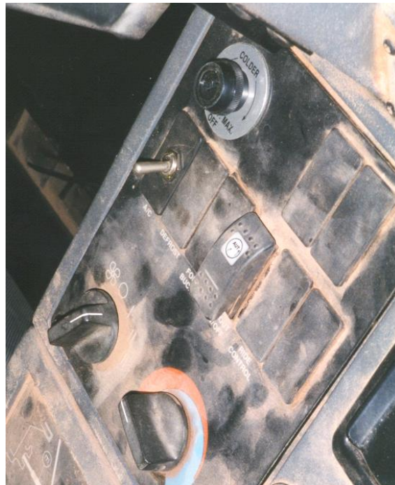
Thermostat location on panel.
